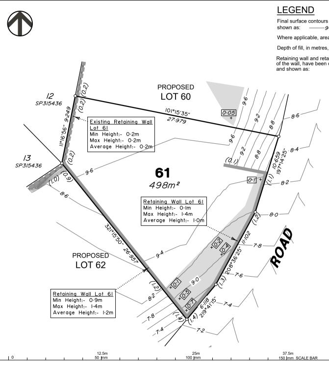
Final surface contours based on A.H.D. datum at an interval of 0.2m. shown as: ——9.5—
