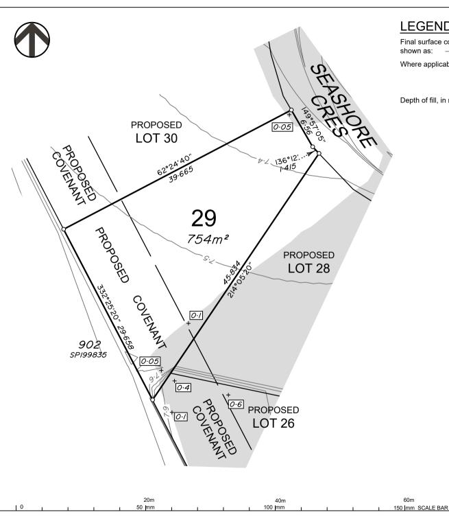
Final surface contours based on A.H.D. datum at an interval of 0.1m, shown as: —— 8·7—
