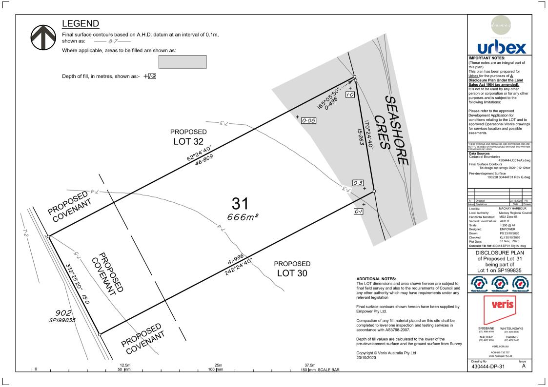
Final surface contours based on A.H.D. datum at an interval of 0.1m, shown as: —— 8-7——
