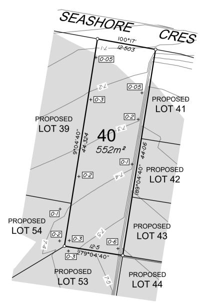
Final surface contours based on A.H.D. datum at an interval of 0.1m, shown as: —— 8·7—
