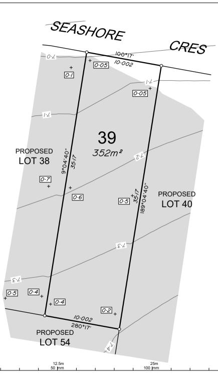
Final surface contours based on A.H.D. datum at an interval of 0.1m, shown as: —— 8·7—
